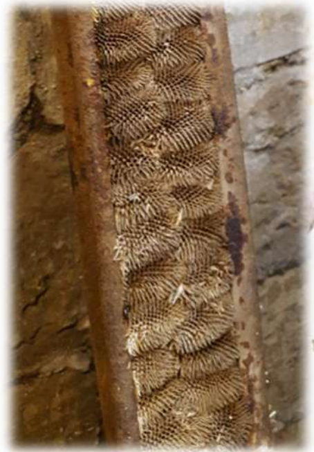
An iron frame from a teasel gig machine at Dunkirk Mill
